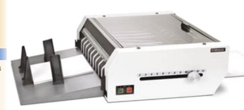
The FD 500 heavy-duty Table Top Burster is a machine to meet almost any forms handling requirement. The FD 500 with side trimmers operates at 90 feet per minute, and can separate one to six-part forms.
