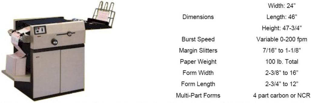
FEATURES: Electronic solid state controls • Automatic jam detection w/ instant braking • Adjustable burster bar • Interlock Safety Cover • Synchronized sequence stacker • Neon "Power On" Switch • High Torque D.C. Motor • Friction-Feed Slitter with Adjustable Side Guides • Heavy Duty Metal Construction • Last Form Shut-Off
