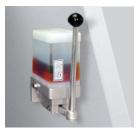
A centralized oiler provides quick and easy lubrication of the cutting head.
